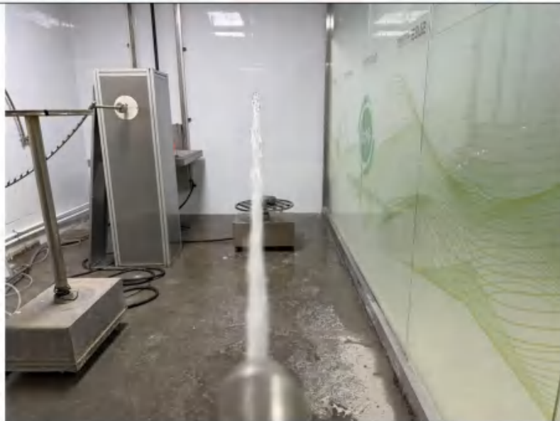
Photo 4: IPX5 test of model AS-GS-FL35-18W
