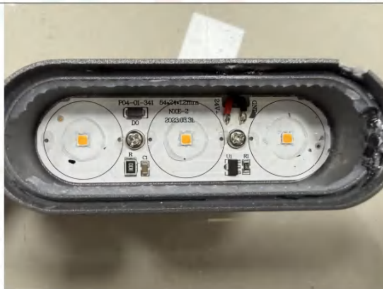
Photo 6: Test result of IP6X and IPX5 test
