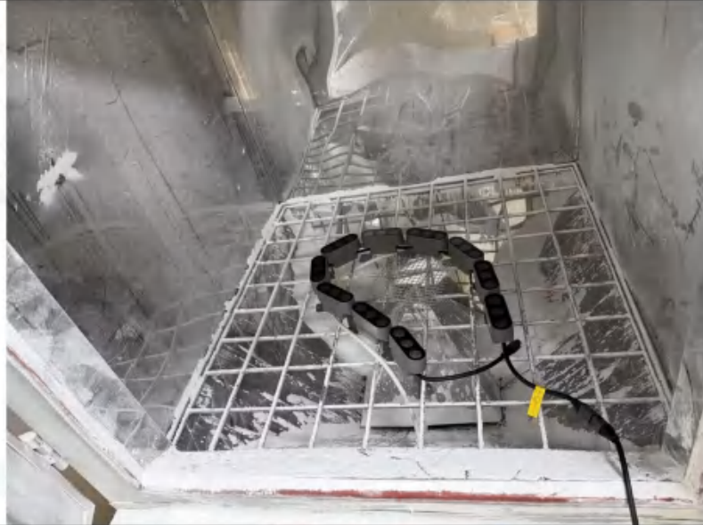
Photo 3: IP6X test of model AS-GS-FL35-18W
