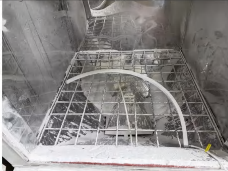
Photo 3: IP6X test of model AS-GS-FN30P6
