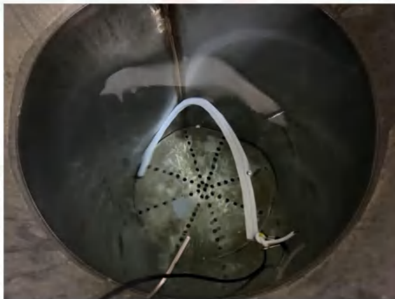
Photo 4: IPX7 test of model AS-GS-FN30P6
