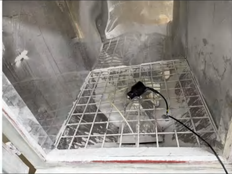
Photo 3: IP6X test of model AS-GS-RS55-1.2W
