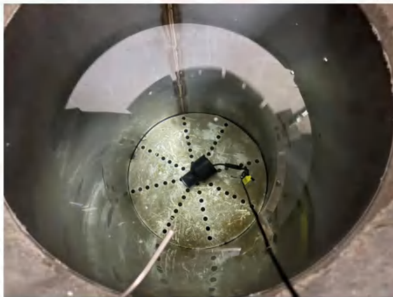
Photo 4: IPX7 test of model AS-GS-RS55-1.2W
