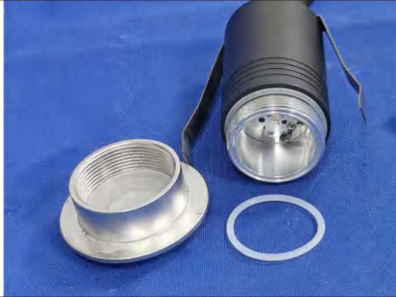
Photo 5: Test result of IP6X and IPX7 test
