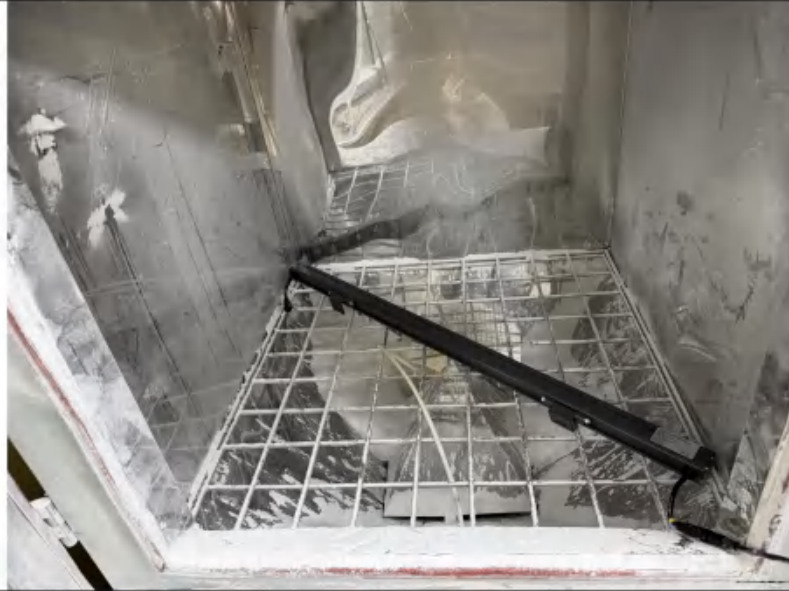
Photo 3: IP6X test of model AS-GS-SW38-13W
