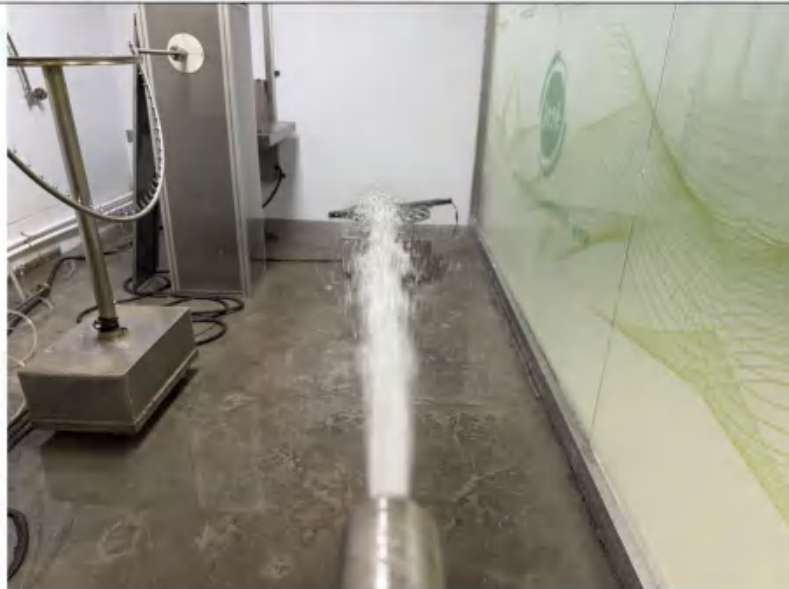
Photo 4: IPX6 test of model AS-GS-SW38-13W
